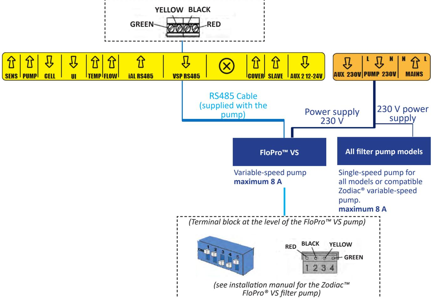
**2.5.6 Connecting to an auxiliary device = AUX 1 - Dry contact provided for disconnection from the 230V power supply**
