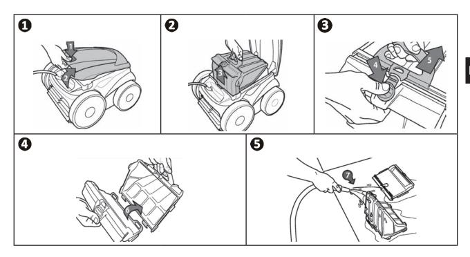
Tip: Check the status of the "filter cleaning" indicator (depending on the model) We recommend that you clean the filter as soon as the LEDs light up.
