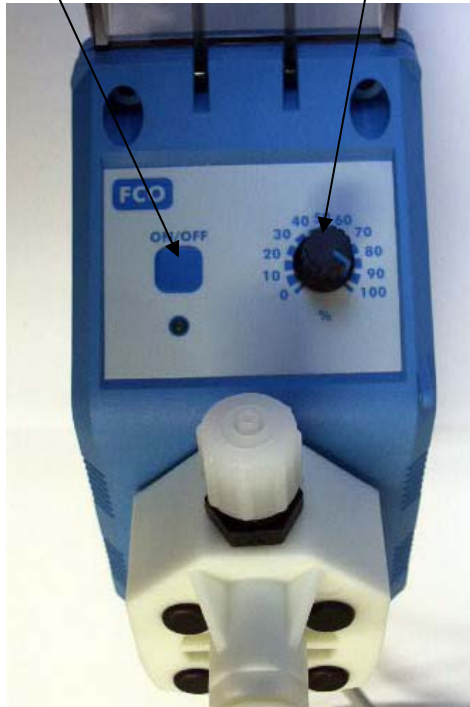
Speed regulator of water dosing or fragancies
