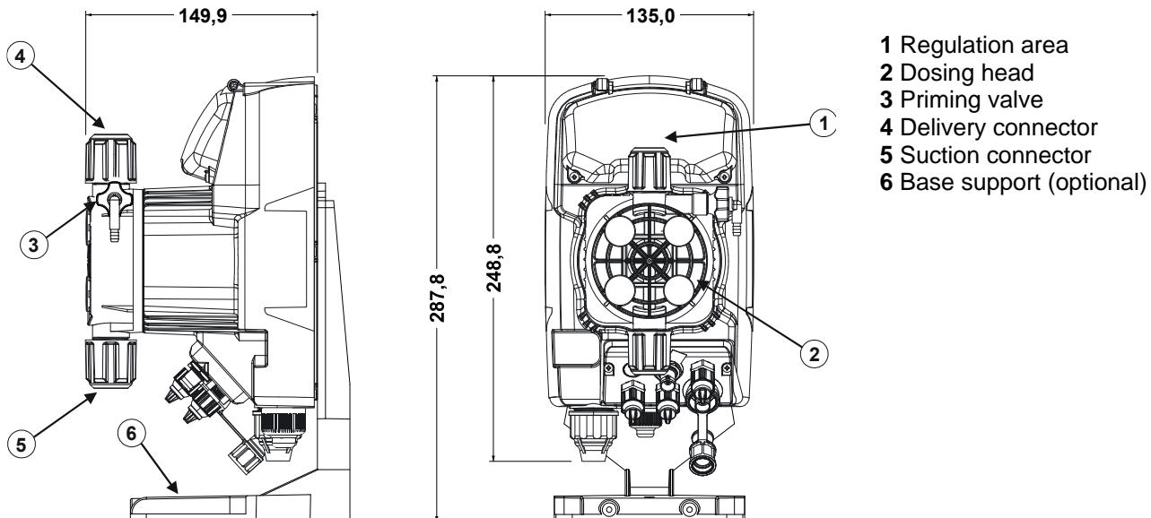
The parts in contact with the liquid have been chosen in order to guarantee perfect compatibility with most chemical products normally in use. Given the range of chemical products available on the market, we recommend checking the chemical compatibility of the dosed product and contact materials.
