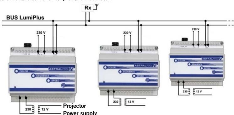
The system can synchronize up to 10 modulators, and a maximum of 3 antennas can be mounted in one installation in order to guarantee maximum coverage.
