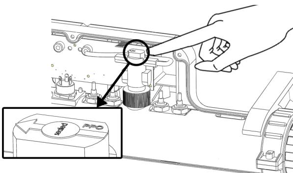
Locate flowswitch. Flow direction is shown by the arrow on top.
