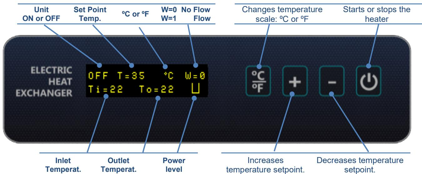
The unit will show if it is heating water by means of this icon on the lower right side of the screen:
