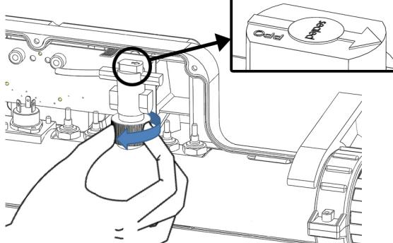
Screw nut back and ensure that it is completely locked to achieve desired watertightness.
