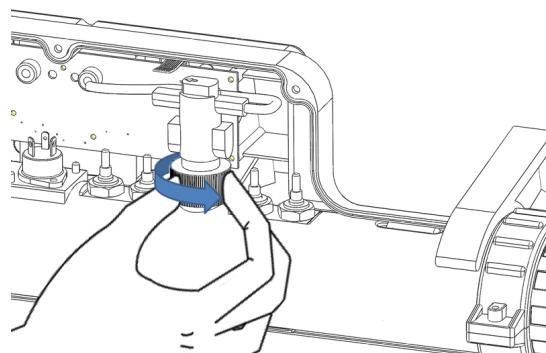
Unscrew nut until flowswitch main part is able to rotate.
