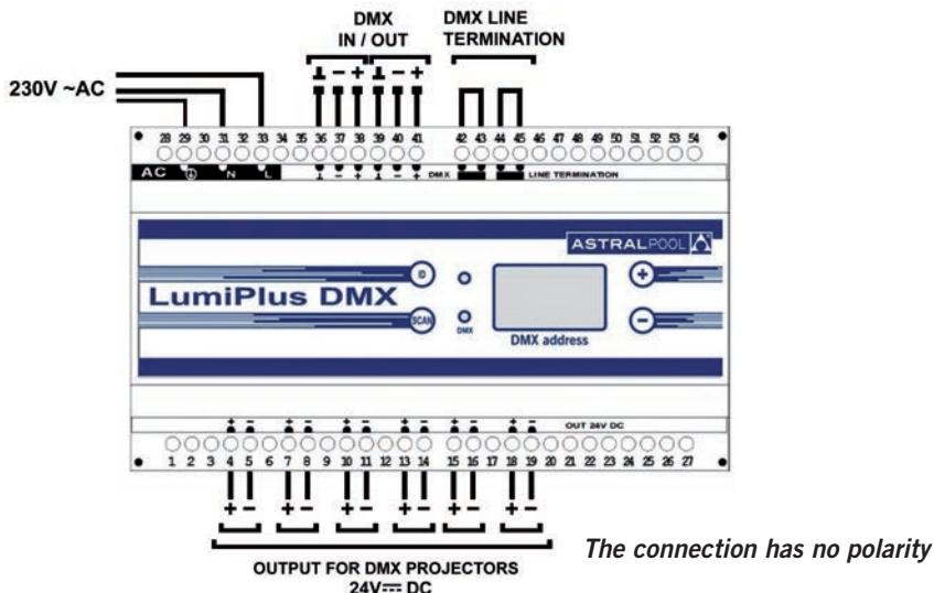
See manual of the DMX mains lead code 52142 for information regarding how to assign DMX addresses to each Mini LED projector and how to configure a system.
