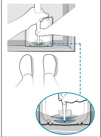
4 Use the handle to take it out of the water. The cleaner expels water through a rear jet to make it lighter
