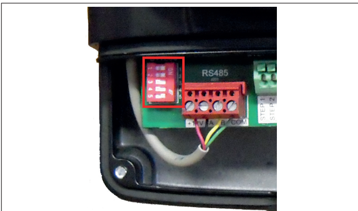
Position of the switches for control via iQPUMP
