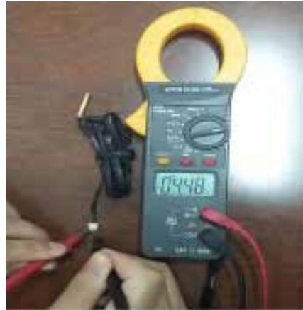
**EN:** Resistance measurement method: power off the unit before testing, turn the multimeter to measure resistance gear KΩ. If the resistance value cannot be measured well, check whether the terminals are in contact or not. If the contact is good, it is judged that the sensor is damaged.
