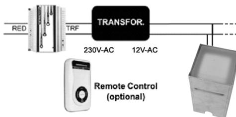
**Each Modulator can control up to a maximum of 90 LED spotlights.**
