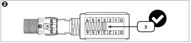
If necessary, use the pool valves to adjust the flow rate so that the indicator light is in position 3.
