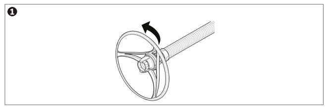
For the T5 Duo model, the quick connector is not integrated into the wheel deflector:
