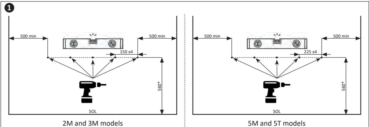
\*Distance to be respected when the dehumidifier is mounted on the base. If this is not the case, this distance can be increased.
