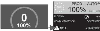
The cell alarm will appear when the devices detect that the electrode is at the end of its life (passivated).
