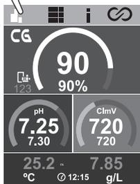
The statistics show a history of the production parameters – pH, ClmV, T – during device operation. You can choose between displaying statistics for the last 24 hours or the last 24 days.
