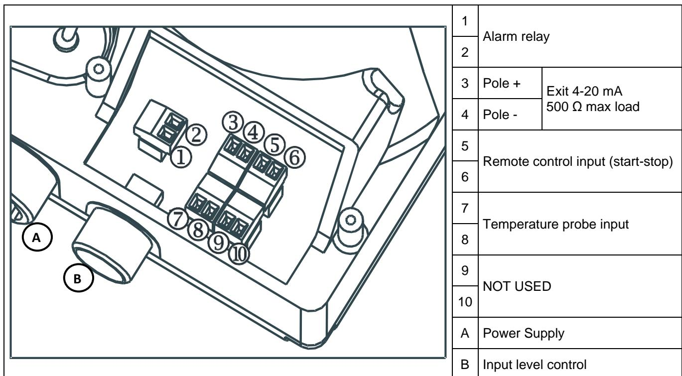
The pump must be connected to a power supply that complies with that indicated on the label on the side of the pump. Failure to respect these limits may cause damage to the pump itself.
