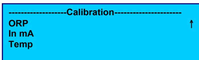
Use the **Up** and **Down** keys to select the probe to be calibrated and press **ENTER**.
