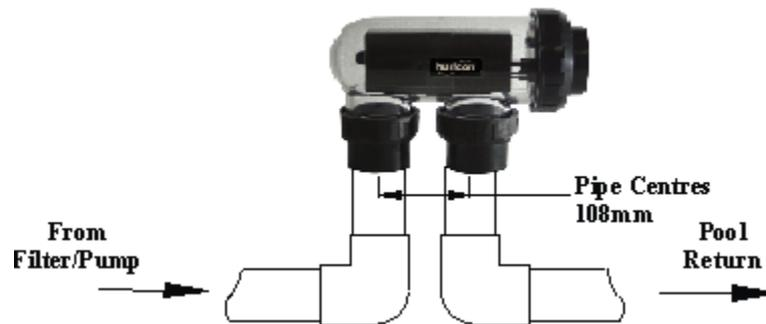
**WARNING:** It is essential that pipe work and equipment do not allow gases generated from the cell to collect and build up.
