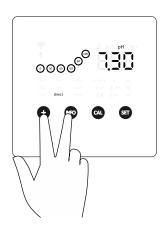
3) Configure the device in pairing mode (hold "+" & "INFO" simultaneously for 5 seconds)
