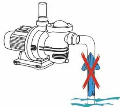
**EN** No water in the prefilter or clogged prefilter.
