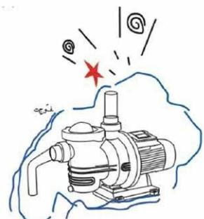
**EN** Low flow rate: low pressure in the filter.
