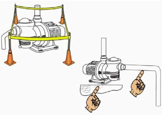
**EN** To avoid problems in suction, make a positive slope of the suction pipe towards the pump.
