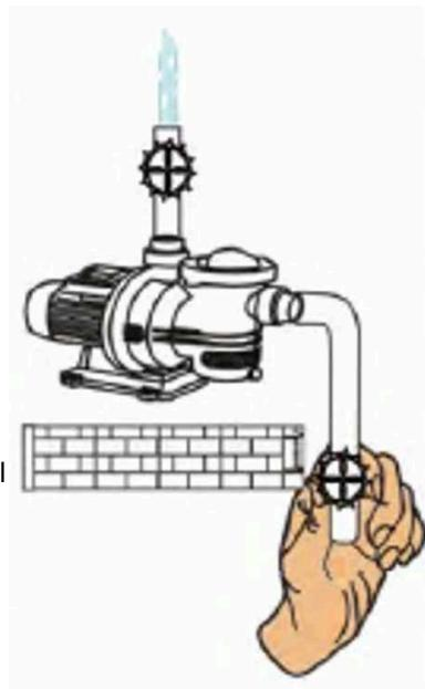
**EN** Fill the pump, slowly and completely opening the gate valve in the suction pipe, and keeping the gate valve on delivery open to let the air out.
