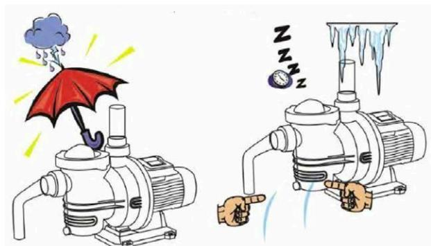
**EN** For long periods of inactivity or frost, remove all the caps and completely drain the pump body. Keep the caps!
