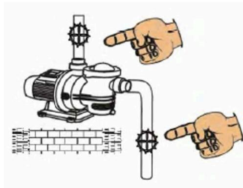
**EN** Fit one gate valve in the suction pipe and one in the delivery pipe to isolate the pump.
