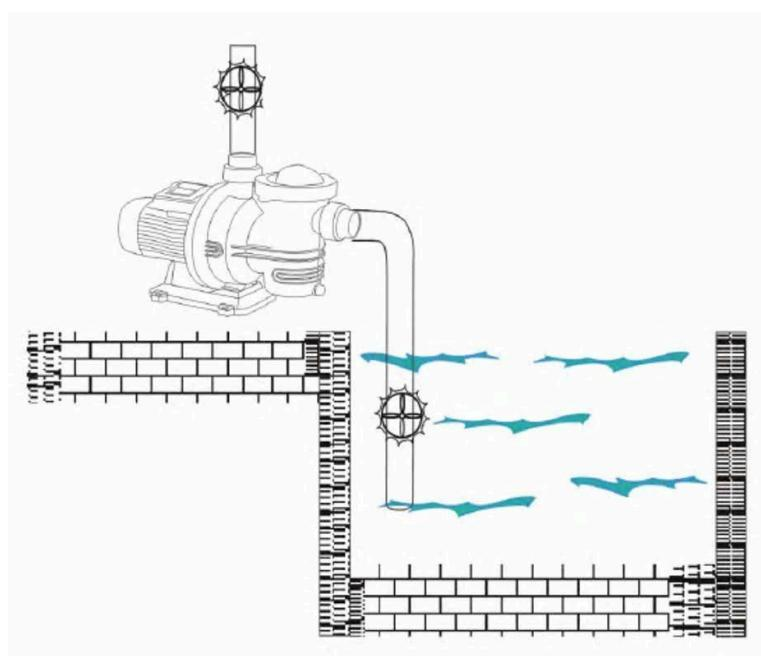
**EN** The pump is able to overcome a maximum difference in level of 1,5 m.
