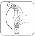
Dissolve tablet(s) by inverting.
