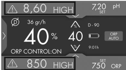
The integrated pH / ORP (mV) controller has an ALARM signal that is activated when an abnormal value outside the range is detected, greater than pH 8.5 / ORP 850. For safety reasons at pH > 8.5 (HIGH) the pH dosage is stopped.
