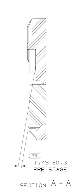
DELIVERY CONDITION TO WIRE ASSEMBLY PLANT fls pre-staged position before terminals
