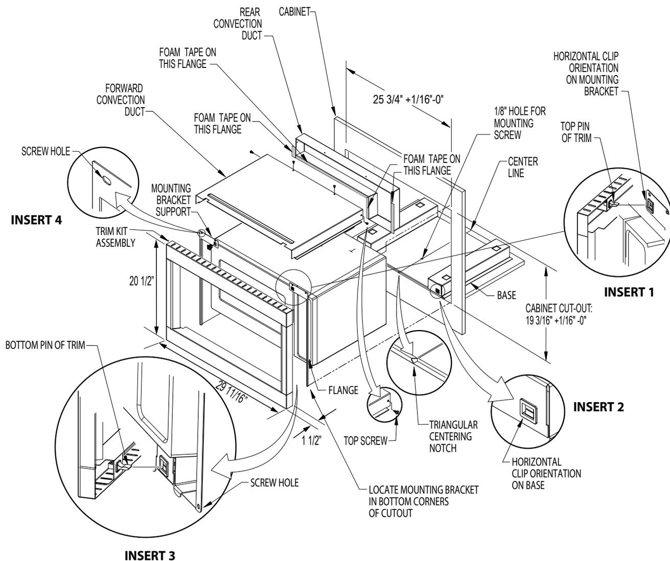
Note: when installed, the trim assembly is positioned symmetrically over the cabinet cut-out
