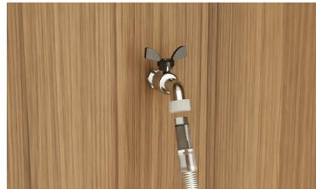
Connect the inlet hose to tap and handtighten into place. Using a spanner or pliers, turn a further 180° to secure. Avoiding over tightening.
