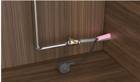
Route the hard wiring through the service hole in the side of the cabinetry.
