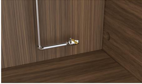
Flush water line into a bucket.
