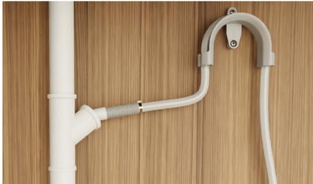
Pull the hose through the drain hose support before threading the hose clamp onto the hose and fitting to the sink trap. Secure to trap using the clamp. Ensure hose is routed straight to the trap.
