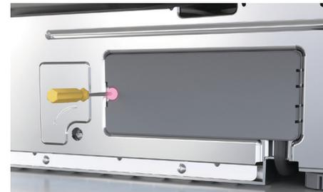
Refit the junction box cover ensuring all wires are clear of the cover. Ensure the power cord is routed under the dishwasher.
