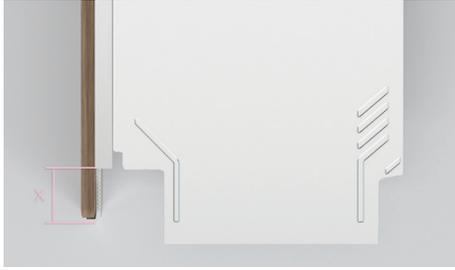
Measure the custom panel overhang from the base of the inner door. Refer to the table below for the recommended cut location.
