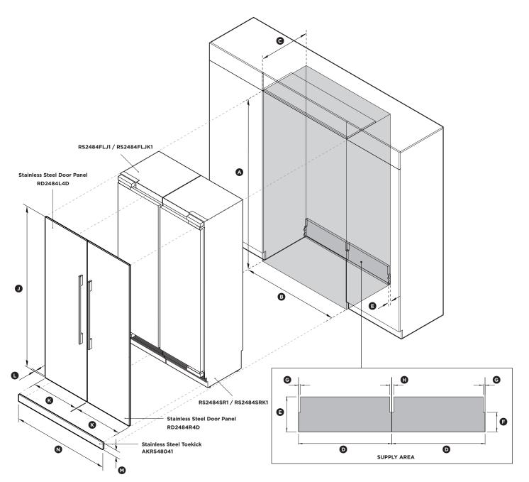
ISO VIEW OF 1219mm CAVITY (610mm + 610mm)
