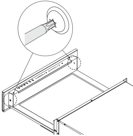
Open the drawer fully, and slightly loosen the T20 star head machine screws.
