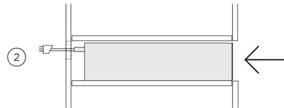
Push the warming drawer back into the cabinetry, and align the flanges with the cabinetry as desired.
