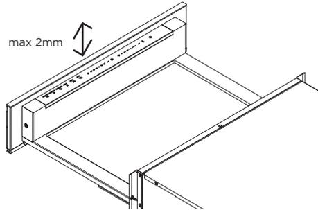
Adjust to the required height and then re-tighten the screws. The height is adjustable within 2mm.
