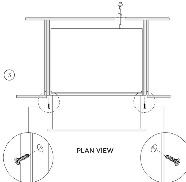
Open the drawer and secure the attachment flanges of the drawer to the side edges of cabinetry with T20 star head machine screws.
