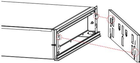
Align the panel to the chassis and slot into place.
