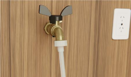
Ensure the rubber washer is fitted when connecting the inlet hose to the tap. Hand-tighten into place. Using a spanner or pliers, turn a further 180° to secure. Avoiding over-tightening. **Do not turn water supply on. The Dishwasher must be powered on for the flood protection feature to be enabled.**
