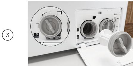
3 Turn the filters anti-clockwise to remove. Clean and rinse each filter. Check and clear the cavity behind each filter. Check the impeller behind each filter moves freely and remove any obstructions.
