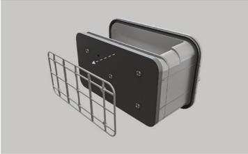
Remove the bracket securing the foam to condenser filter.
