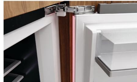
Locate the shorter door trim to the hinge-side of the product, and slide down to clip in place. If a gap is present, remove and readjust the side brackets. Repeat for lower door.
