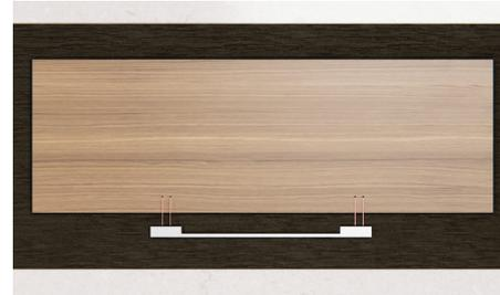
Ensure all bracket and handle holes have been pre-drilled. Refer to 'custom panel preparation' for details.
