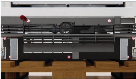
Push the grille flap to open and unscrew the two screws behind the flap and five on the grille. Set screws aside. Open the door and pull the grille outwards from the product.
