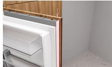
Locate the longer door trim to the non-hinge-side of the product and slide down to clip in place. If a gap is present, remove and readjust the side brackets. Ensure trim does not protrude above the top cover. Repeat for lower door.
