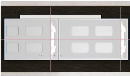
Align the centre bracket to pre-drilled holes on the panel.
