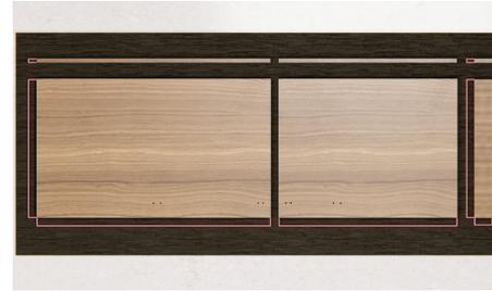
Ensure all door and toe kick panels are square and set up to the correct specifications. Refer to 'custom panel preparation' for details.
