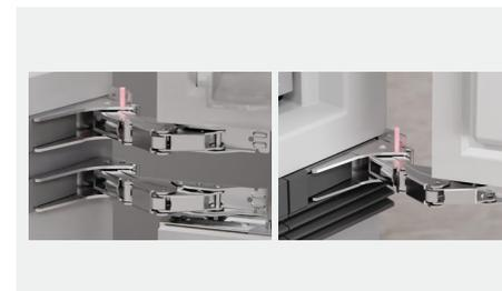
To limit the door opening to 90°, place the hinge limiting pin into the lower hinges on both doors.
