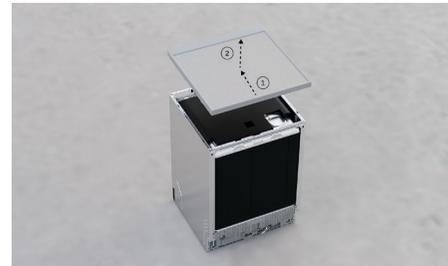
Slide forward 20-30mm, then lift upwards. Ensure moisture tape is installed if removing top panel.
