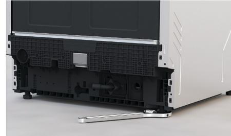
Using a spanner, level the rear legs first followed by the front legs. Clockwise to raise the height, anticlockwise to lower the height.
