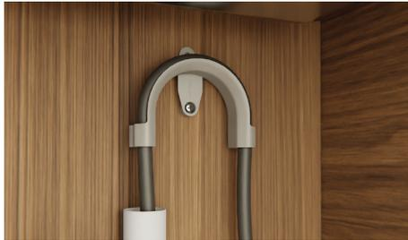
Pull the hose through the support guide and rest in standpipe. Ensure the drain hose does not extend into water retained in the trap; an air gap is required to prevent waste water from siphoning back into the tub.
