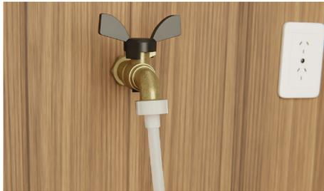
Ensure the rubber washer is fitted to the coupling before connecting the inlet hose to the tap. Hand-tighten into place. Using a spanner or pliers, turn a further 180° to secure. Avoiding over-tightening. **Do not turn water supply on. The Dishwasher must be powered on for the flood protection feature to be enabled.**
