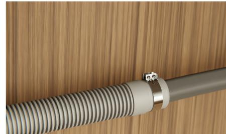
Pull the hose through the drain hose support before threading the wire clip onto the hose and fitting to the supplied hose joiner. Secure using the wire clips. Ensure hose is routed straight to the joiner, remove any excess drain hose.
