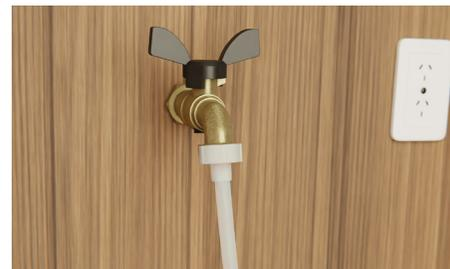
Ensure the rubber washer is fitted to the coupling before connecting the inlet hose to the tap. Hand-tighten into place. Using a spanner or pliers, turn a further 180° to secure. Avoiding over-tightening. **Do not turn water supply on. The Dishwasher must be powered on for the flood protection feature to be enabled.**
