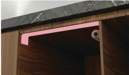
Align the supplied moisture protection tape to the cabinetry as shown. Ensure this area is free of debris before carefully applying the tape to the surface.
