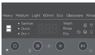
Press and hold » until a tone sounds. When
