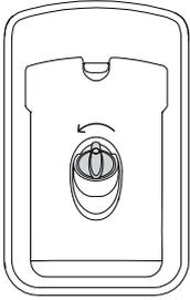
Turn the plug anticlockwise and remove.
