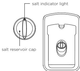
The salt reservoir is located on the inside of each drawer next to the detergent dispenser. It holds up to approximately 350g of salt (actual capacity will vary depending on brand and grain size of salt used).
