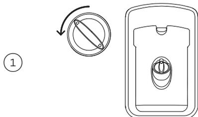
Turn the cap anticlockwise and remove.
