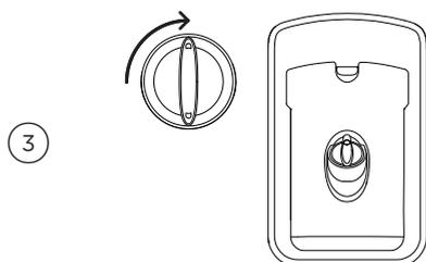
Refit the cap, turning clockwise until secure.
