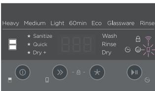
If the drawer is open,
