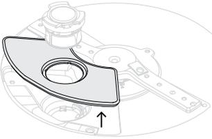
With the drain filter removed, carefully lift the drain filter plate up and out. Clean under hot soapy water and rinse thoroughly.
