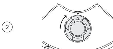
Push the drain filter back into the tub and rotate clockwise until the arrows on the filter and base of the drawer align.
