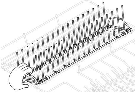
Slide the tines backward or forward by pushing or pulling the front handle.
