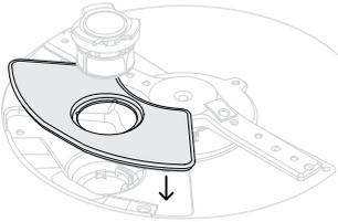
Push the drain filter plate back onto the tub ensuring there are no particles in the recess.
