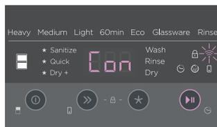
Press and hold **▶▶** to connect to the Wi-Fi network.
