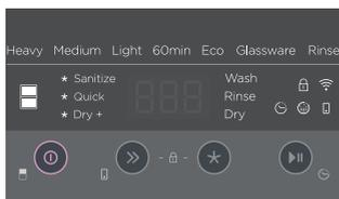
Press and hold **⏻** to save and leave the menu after Wi-Fi is connected.
