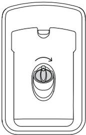
Refit the plug, turning clockwise until secure.
