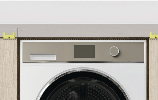
2. Check alignment and ensure required clearances are maintained. Adjust as required.
