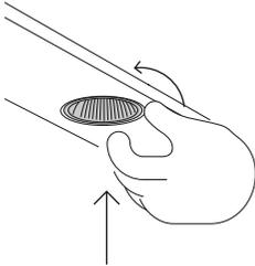
Lightly push the light bulb up and rotate anti-clockwise to remove.
