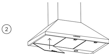
Place the filter into the support at the rear of the rangehood. Push the filter back into place.
