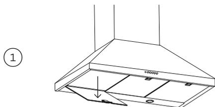
Pull the catch and tilt the filter downwards until it disengages from the supports.
