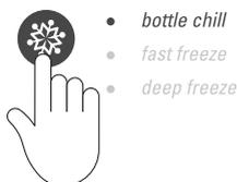
This feature allows you to rapidly chill your beverages in the freezer without the worry of forgetting about them. An alarm will sound and the 'bottle chill' light will illuminate after 15 minutes to remind you to remove your beverage. Remember to remove your beverage when the alarm sounds, to ensure the liquid does not freeze.
