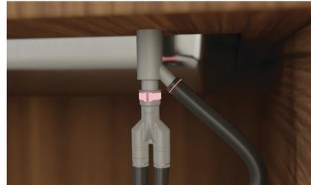
Thread wire clip on to the hose before fitting hose to the supplied hose joiner. Secure using the hose clamps. Fit to the Air Gap Kit. Ensure hose is routed straight to the joiner, remove any excess drain hose. Unplug or drill out the waste tee before securing to sink trap or waste tee.
