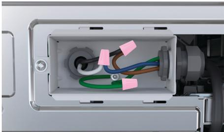
Install the strain relief into the junction box bracket and secure the house wiring or the power cord and tighten. Thread the wires through the hole in the junction box bracket and connect the incoming ground to green, white to white and black to black.
