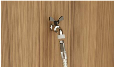
Connect the inlet hose to tap and handtighten into place. Using a spanner or pliers, turn a further 180° to secure. Avoiding over tightening. **Do not turn water supply on. The dishwasher must be powered on for the flood protection feature to be enabled.**
