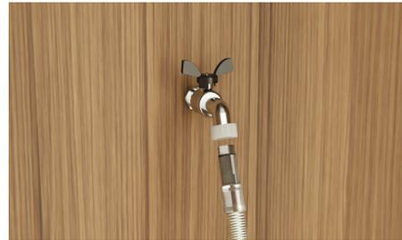
Connect the inlet hose to tap and handtighten into place. Using a spanner or pliers, turn a further 180° to secure. Avoiding over tightening. **Do not turn water supply on. The dishwasher must be powered on for the flood protection feature to be enabled.**
