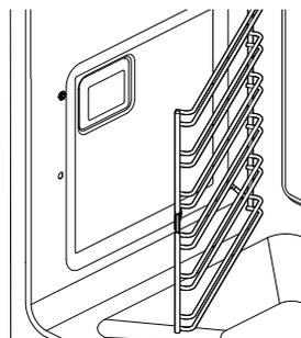
Slide the side rack forward until the rear prongs are clear of the holes.
