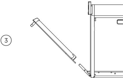
Holding the door on both sides, lift door back up to 45° and carefully pull the door out and away from the hinges.
