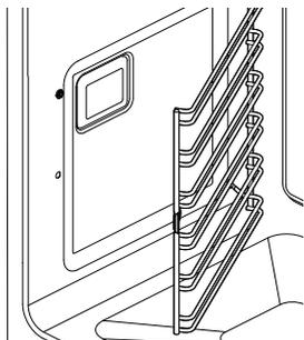
Slide the rear prongs of the side rack back into the holes, ensuring the rack is firmly pushed up against the side wall of the oven.
