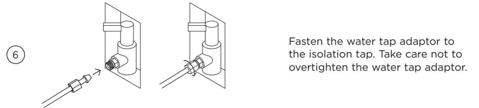
Fasten the water tap adaptor to the isolation tap. Take care not to overtighten the water tap adaptor.
