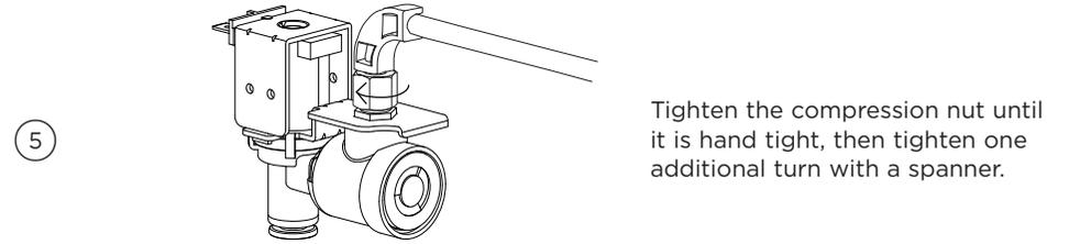
Tighten the compression nut until it is hand tight, then tighten one additional turn with a spanner.
