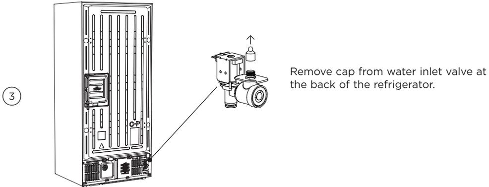
Remove cap from water inlet valve at the back of the refrigerator.
