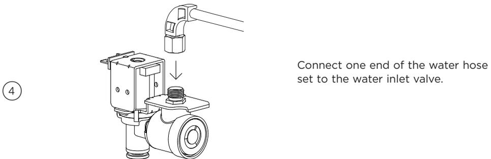
Connect one end of the water hose set to the water inlet valve.
