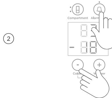
Press the , , and together for 4 seconds then close the doors. The ice tray will empty the water into the bin below. The ice tray will only empty after the doors are closed.
