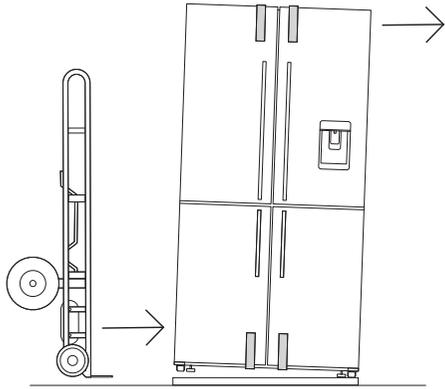
Tilt the appliance slightly forward and insert the hand truck between the pallet and appliance.
