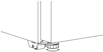
Adjust the front feet down until the refrigerator is leaning backward with the front approximately 10mm higher than the back. This will ensure a good door closing action.
