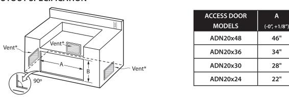
NOTE: The cutout of each corner should be 90° angle in order for the access doors to fit properly. \* Island installation to use minimum of 3 vents providing 10 sq. in. per vent (typical).
