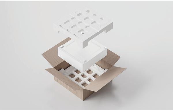
2. Cut the straps and tape to open the plinth carton from the top. Remove the EPS cap before lifting the plinth out.
