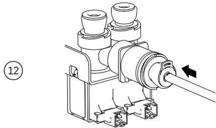
Insert the outlet tubing to water (solenoid) valve up to the marked line.
