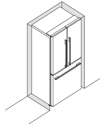
Roll the refrigerator back into position and adjust front feet. Check alignment and door closing action are satisfactory. Make small adjustments to the front feet where necessary.
