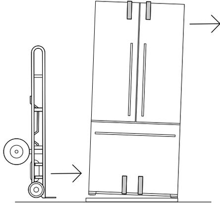
Tilt the appliance slightly forward and insert the hand truck between pallet and appliance.
