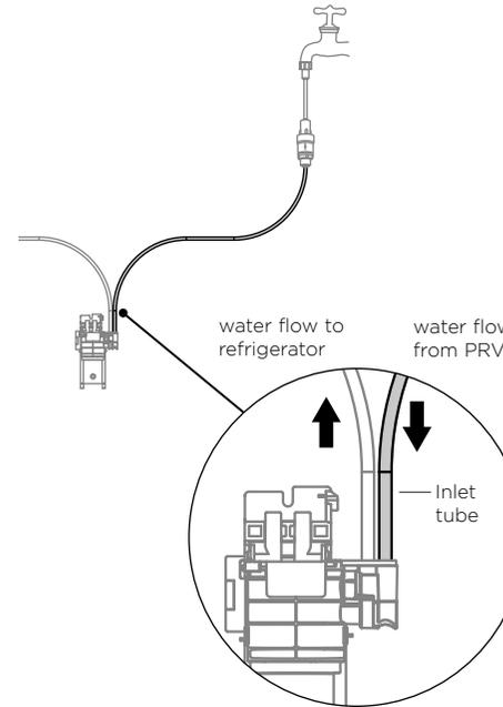
Connect the inlet tube from the filter head to the PRV. The inlet tube can be identified by the downward arrow ↓ on the filter head and a red mark on the tube.
