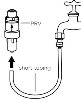
Connect the inlet of the PRV to the tubing connected to the faucet. Ensure the arrow on the PRV is pointing away from the faucet. The arrow indicates the direction of water flow.
