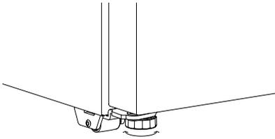
Adjust the front feet down until the refrigerator is leaning backward with the front approximately 3/8" 10mm higher than the back. This will ensure a good door closing action.
