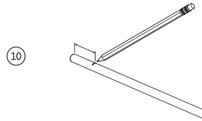
Measure 5/8" (16mm) from one end of outlet tubing and mark a line.
