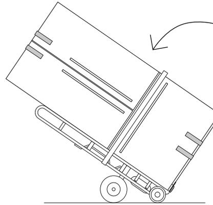
Tilt backward to load appliance onto hand truck and push to install location.
