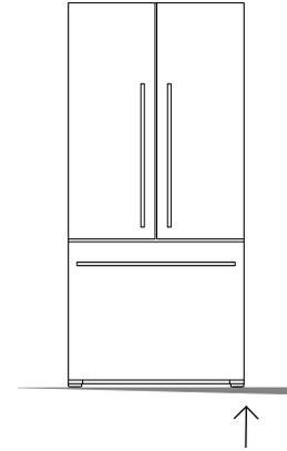
Gently push the refrigerator back until the rear rollers contact the floor.
