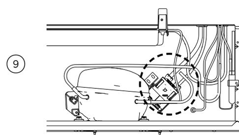
Run the 1/4" (6mm) tubing to the back of the refrigerator ensuring there is enough tubing to pull the refrigerator out for service.
