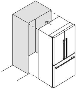
Roll the refrigerator into its final position ensuring there is the correct air gap between the product and surrounding cabinetry. See minimum clearance in cabinetry dimensions table.
