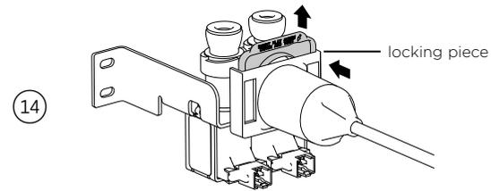
Slide the cover all the way through the water valve. Pull up the locking piece and push the cover until it snap-locks into the valve.
