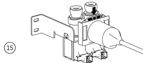
Check if the cover is aligned correctly. Press the locking piece down to lock the cover in place.
