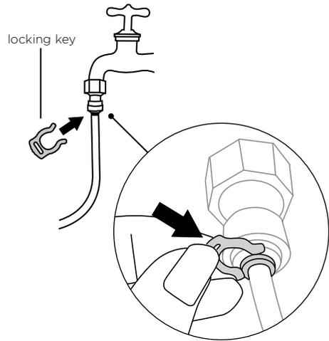
Connect the short tubing to the outlet of the faucet and secure with the locking key.
