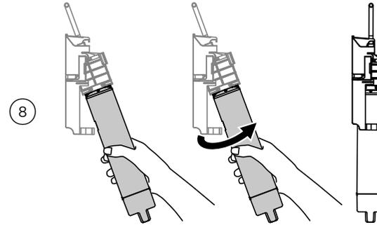
Insert the filter water into the filter head. Push the filter firmly into the filter head and turn in a clockwise direction until it locks into place.
