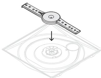
Place the spray arm onto the impeller. Ensure that the arm rotates freely when refitted.
