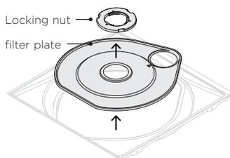
With the filter and spray arm removed, twist the locking nut anti-clockwise and lift out. Carefully lift the filter plate out and clean under hot soapy water before rinsing thoroughly.
