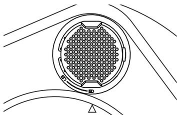
Place the filter back into the tub by aligning the arrow to the
