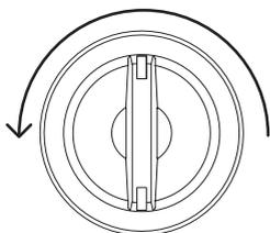
Turn the cap anticlockwise to remove.
