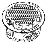
Align the filter cap with the notch on the filter base. Click together to secure.
