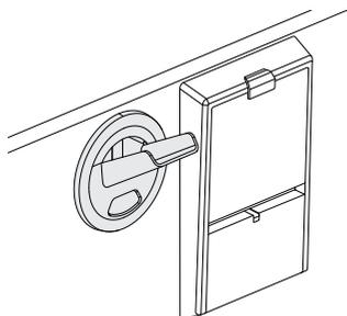
Attach the salt funnel to the DishDrawer™ Dishwasher and carefully pour salt into the reservoir.
