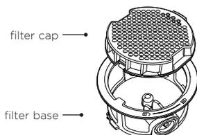
Separate the filter cap from the filter base by pressing the release button and lifting.
