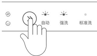
Press » to change the setting within an option. The wash program indicators will display which setting is selected. Refer to 'Settings display' for details.
