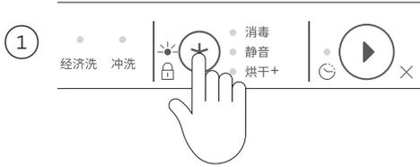
Open the Dishwasher and press and hold ★ until a tone sounds and the lock indicator begins flashing.
