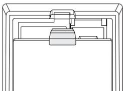
Press the latch down to open the dispenser before lifting the rinse aid cover.
