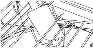
Ensure the spray arm can rotate freely and there are no protrusions below the rack.
