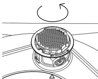
Twist the filter counter-clockwise until the arrow in the tub points to
