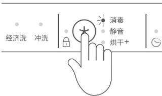
Press ★ to scroll through the settings. The wash modifier indicators will display which setting is selected. Refer to 'Settings display' for details.
