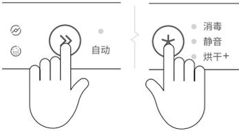
Ensure there is no wash in progress, then open the drawer. Press and hold » and ★ together for four seconds.
