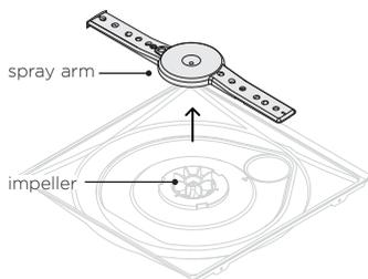
Lift the spray arm off the impeller, pulling up from the centre. Shake to dislodge any loose particles, rinse under running water and wipe with a damp cloth. Ensure the magnet is clean and clear and that water can flow through all holes.
