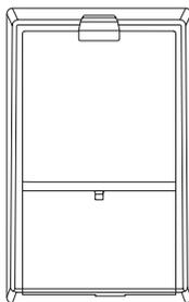
The salt reservoir is located on the inside of the drawer next to the detergent dispenser. It holds up to approximately 400g of salt (actual capacity will vary depending on brand and grain size of salt used).
