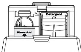
Lift the cover open and pour rinse aid into the opening taking care not to spill any into the drawer or detergent bucket.
