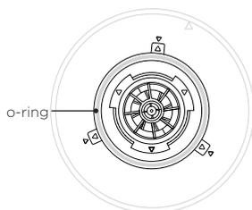
Before refitting the filter plate, ensure the O-ring is correctly positioned in the tub as shown.
