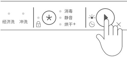
Press and hold ►, each tone indicates + 1 hour delay and can be set for up to 12 hours.
