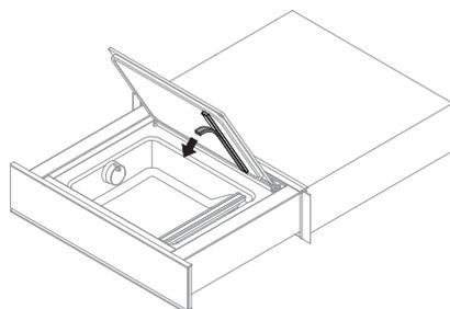
The seal pad is located on the underside of the drawer lid.
