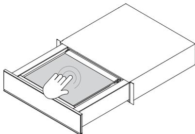
Before pressing the play button ▶, hold down the lid so the gasket forms a seal with the product.
