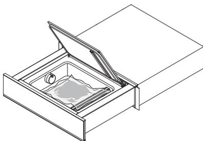
Place the food inside the vacuum bag. Open the glass lid and place the bag inside the drawer. Secure the opening of the bag under the bag clip and position across the sealing bar.
