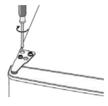
5. Insert the hinge bracket and screw it to the top of the unit. Tighten using a spanner if necessary.
