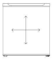
4. Refit the door ensuring it is aligned horizontally and vertically. Check that the gasket is sealing on all sides. Tighten the top hinge.
