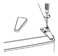
**2.** Remove the top right hinge cover. Unscrew screws from hinge bracket.
