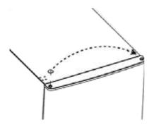
1. Move the cover from the left side to right side before removing the door and placing it on a protected surface.
