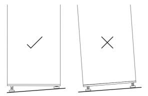
1. Adjust the two levelling feet at the front of the unit so that it is level.
