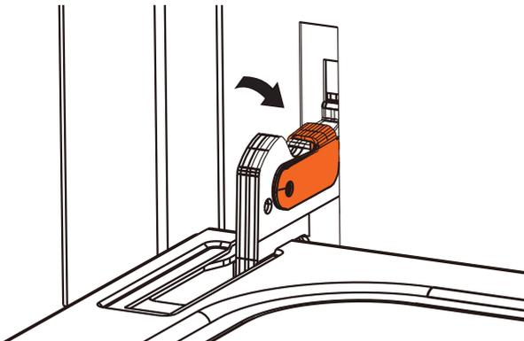
1. Insert the door hinge notches into the slots in the frame of the oven. Push the safety catches down on the hinges before you close the door.
