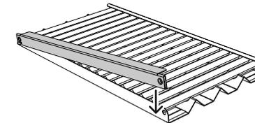
Lock radiant end cap and place the assembled radiant into the unit.
