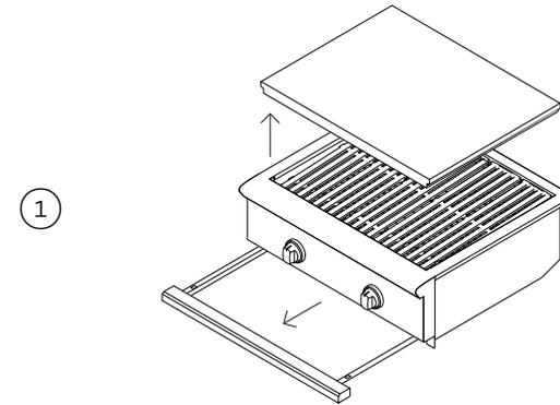
Remove the drip pan and any other removable components from the grill.
