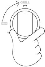
Prepare soap solution by combining one part liquid detergent and one part water. Pour into a spray bottle. Ensure all control valves are in the **OFF** position before turning the gas supply **ON**.
