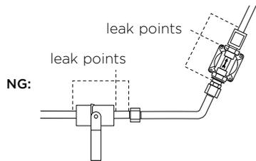
Check all connections from the supply line or LP cylinder by applying the solution around the connection, tubing and end of the manifold. Soap bubbles will appear where a leak is present.
