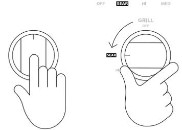
Push in and hold the selected dial for 2 seconds before turning to **SEAR**. Hold for 10 seconds to light the selected burner.
