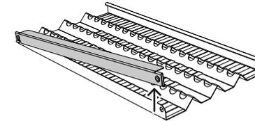
Unlock radiant end cap by pushing it up with two fingers.
