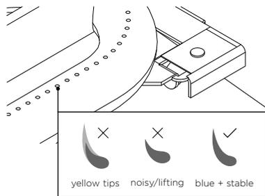
Reinstall the U-burner and light to check. If the flame is blue and stable, remove the burner, tighten the air shutter screw and replace all parts. If flame is still unstable, repeat the above steps.
