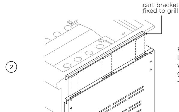
Place the grill head on the cart by locating the rear side tabs of the grill with the slots on the cart. Lower the grill and locate the remaining tabs. The grill should sit flush on the cart.
