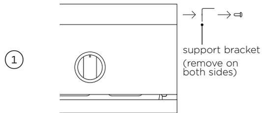
Remove the support brackets from the sides of the grill and replace with the supplied cart mount brackets.
