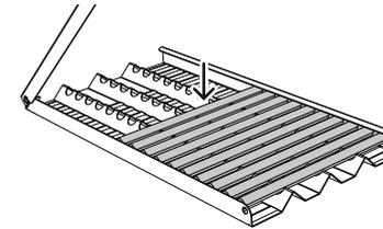
Place all ceramic rods onto the radiant.
