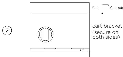
Secure cart mounting brackets using four of the supplied 10-24 x 1/2" screws on each side.
