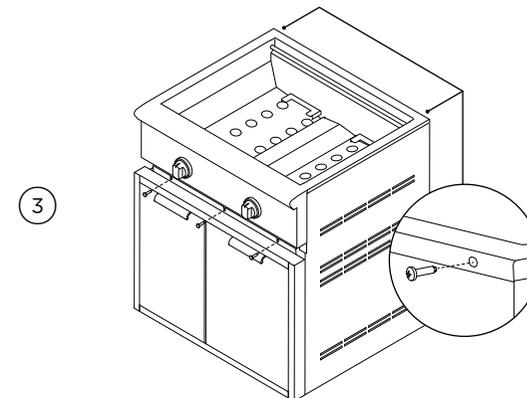
Secure the grill to the cart with two Phillips-head screws at the rear and three at the front.
