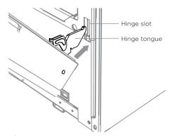
② Align the hinge tongue with the hinge slots and push the door until you feel the latches locate into position on each side.
