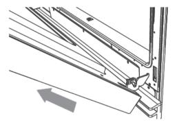
① Disengage the hinges and remove the door. Place on a protected surface.
