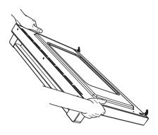
① Hold the door firmly in an approximately halfway open position.
