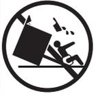
To reduce the risk of tipping the appliance, it must be secured by properly installed anti-tip device packed with the appliance.
