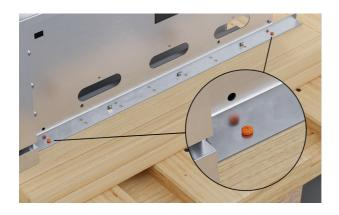
**5.** Remove the two Phillips screws securing the transit brackets to the pallet.
