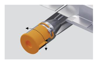
2. Using a Phillips screwdriver, loosen the burner shutter screw and turn shutter to desired position.
