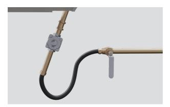
**3. Natural gas must** be connected by an authorized technician.
