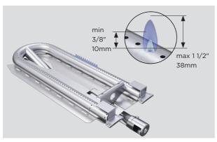
3. Flames should be blue and stable. A yellow flame indicates insufficient air. A noisy flame that lifts away from the burner indicates too much air.
