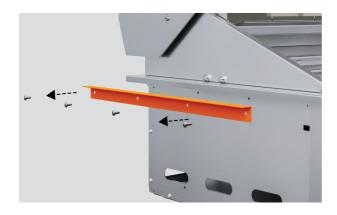
1. Remove the four Phillips head screws at each side of the grill and discard the existing brackets.
