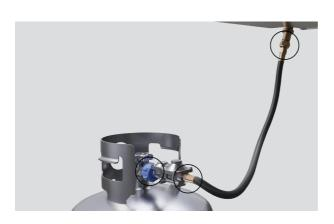
2. Apply a soap solution of 1:1 liquid soap and water to all connections, hoses and fittings from the cylinder to the connection at the grill.
