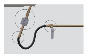
3. If a leak is present, immediately turn off the gas supply, tighten any leaking connections and re-check. If you cannot stop a gas leak, turn off the gas supply and call your local gas utility, or the dealer you purchased the appliance from.
