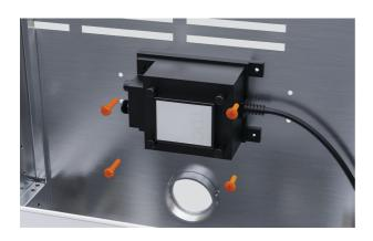
**2.** Screw the transformer into the back of the cart.
