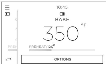
When the oven has reached the set temperature the heating bar onscreen will disappear.
