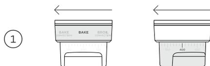
Set the oven to **BAKE** at 400°F (200°C) and heat for 30 minutes.
