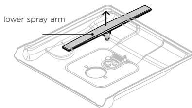
To remove the lower spray arm, lift it from the base of the dishwasher.
